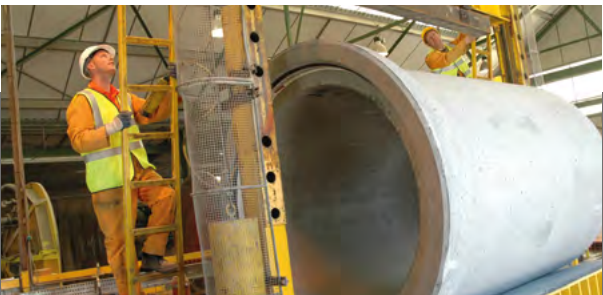
Testing a 1200mm pipe for strength.
